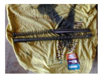
Picture shows the stock spring, spring seat (not always existent) and spacer on top and the progressive WIRTH-spring and stock spacer cut down on bottom. You re-use your stock spring seat. Notice how much longer and thicker the WIRTHs are compared to stock.
