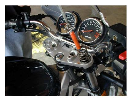
The stock fork spring are sometimes very short compared to the WIRTH-springs. You will need to fish the spring and the spring seat out with either a bent wire (like a clothes hanger-just be careful not to scratch the inside surface of the fork) or you can use an extended magnet, like shown in picture - much easier. The spring seat will be sitting on top of spring and is a seat for the spacer. This comes out too.
