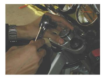
Using a drive socket wrench without a socket or other necessary tool, remove the fork cap bolt and attached o-ring (see photo). <u>There is usually a little spring tension</u> so be careful – best is to put a thick cloth on and around the gas tank. The cap sometimes requires a special tool for removal but wrench sockets often fit perfectly. At this point you can see the top of the stock spacer. Remove it.
